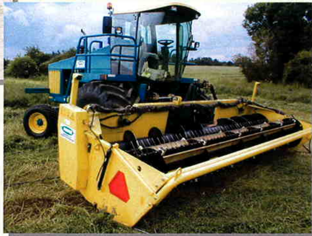
Champion windrover with 6,1m direct cut header single knife double stroke for alfa alfa.
