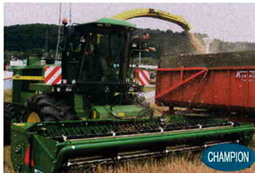
Double knife Busatis Bix and adjustable reel-speed to obtain maximum forward speed and perfect cut and regrowth.
