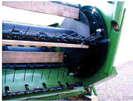
Closed cam track with wide bearings.
