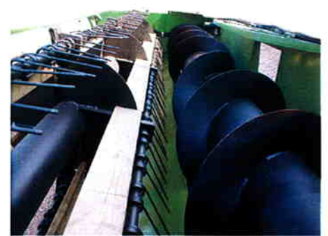
6,0 m/m heavy duty reel tines
